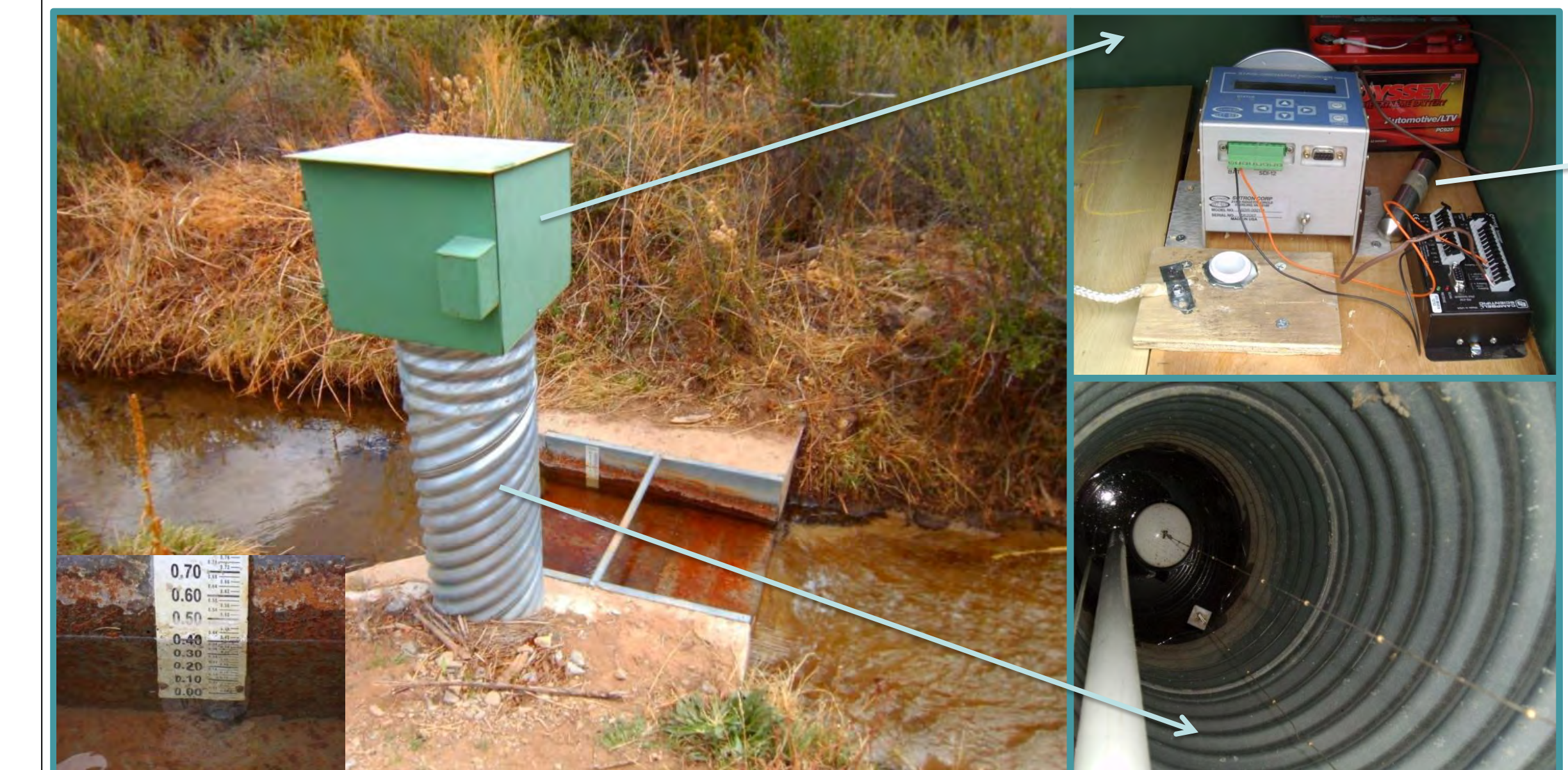
A flume used to measure surface water discharge automatically (Above Left/Inset). A Stage Discharge Recorder (SDR) and data logger are used to record data automatically (Above Top Right). Inside of the stilling well; SDR float and cable (Above Bottom Left)
