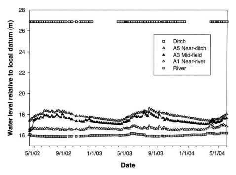
**Figure 3.** Response of shallow groundwater to seepage from irrigation ditch and flood irrigation at the Alcalde Science Center from 2002–2004 shown by: average water level in the Alcalde Ditch; water levels measured in three wells along a single transect (A); and estimated surface water level in the Rio Grande.
