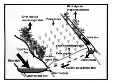
**Figure 4.** Components of hydrologic budget emphasizing surface water–groundwater interactions along irrigated corridor between unlined irrigation ditch and river; arrow widths are related to hypothesized magnitudes of irrigation season fluxes.
