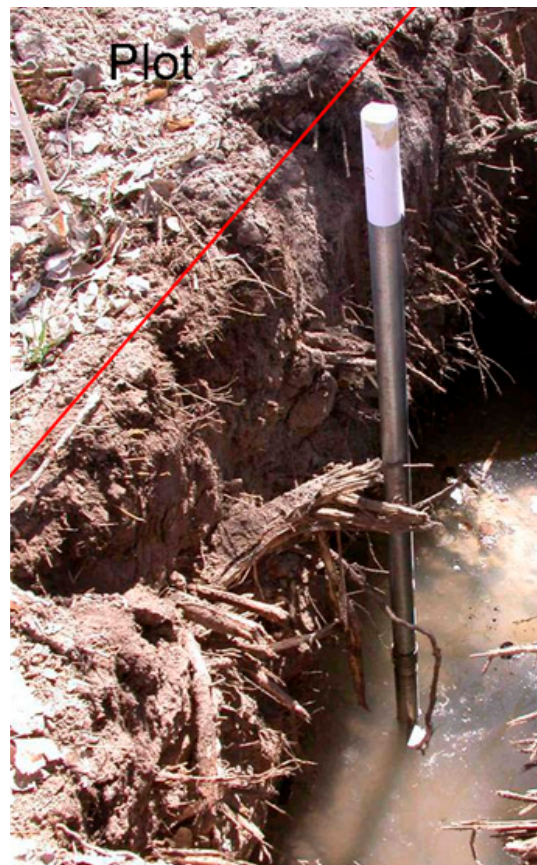
FIG. 10. Photo taken during the north-side well installation in Plot 5, showing a very dense rooting system beneath the surface of the plot.
